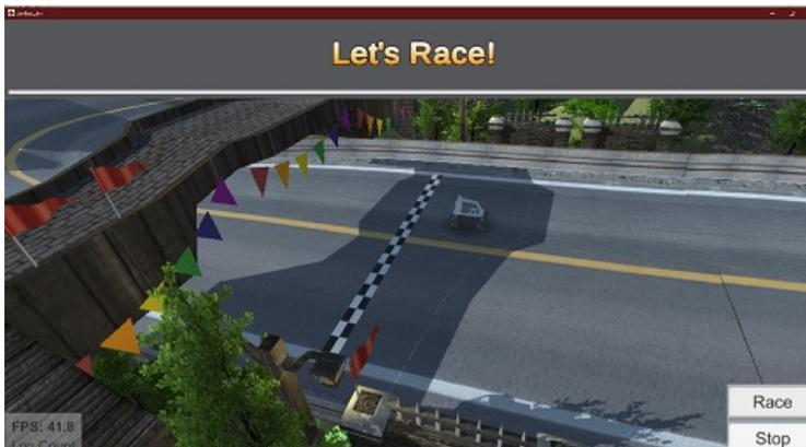
Donkey Car is a high-level, self-driving library written in python. It was developed with a focus on enabling fast experimentation and easy contribution. It typically utilizes a physical R/C car and associated controller to acquire images and data to train a self-driving model. In recent months due to the COVID-19 pandemic, the community developed a simulator to provide the necessary
